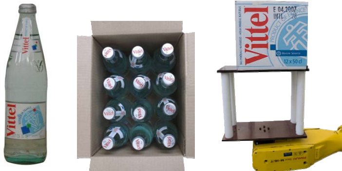
Fig. 11. A photo of one of the 50cl Vitell bottles (left), the inside of the box of Vitell under test, and robot end-effector mounting details for the box
