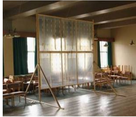
Fig. 1. The frame which supported the grid of tags was constructed of wood, with plastic overlaid for rigidity, and a sheet of thin plastic to which the tags were attached. The wooden chairs behind the frame in the photo were assumed to have negligible effect on RFID operation.
