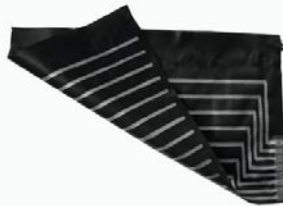
Fig. 3. Conductive silver leads run in parallel across the flexible polyolefin foam to form the 96 sensors. When multiplexed, the leads on different sides of the foam form the capacitive elements.
